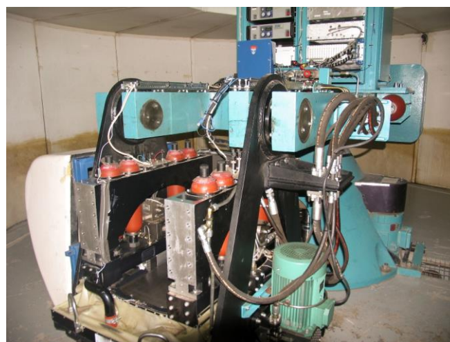
Figure 2. Photo of the UoD centrifuge-mounted earthquake simulator.
